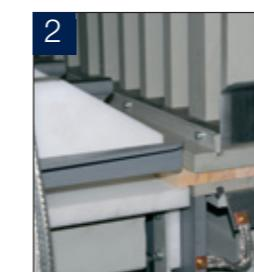
Leaving the glue applicator, the lamellas are cross conveyed into a magazine in which they are gathered in a charge. When the magazine is full, the lamellas are led to a feeding table in front of the press.
