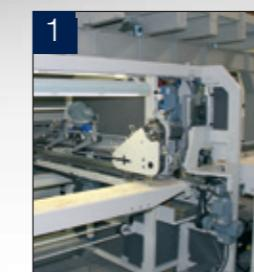
The lamellas pass through the glue applicator one by one. The glue is applied either on top of the lamella by means of a glue nozzle or on the side of the lamella by means of a glue roller, depending on the chosen solution – which again depends on the lamella dimension and your needs.
