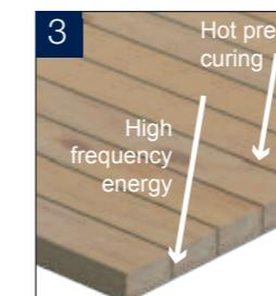
The high-frequency energy targets the liquid in the glue which quickly heats up from the inside and cures.
