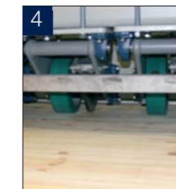
Behind the press, saws can be installed enabling the cutting of the endless board into smaller units – both in longitudinal and transverse directions.
