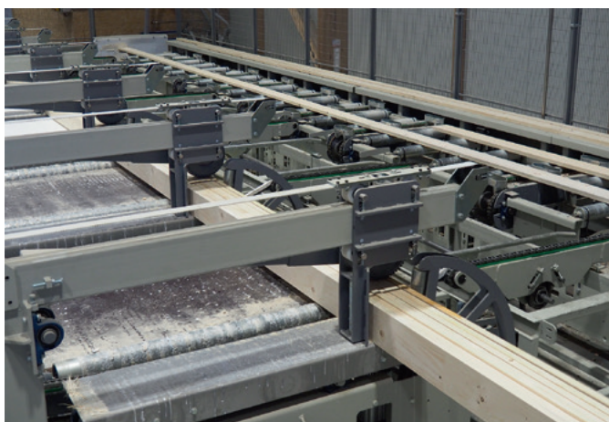
Truss forming: The mechanization by Kallesoe tilts the glued boards that come from the cross conveyor by 90° and this way packages are formed
