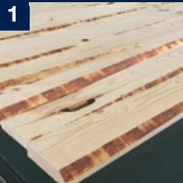
**1** The system can measure the angles of the wane timber and from this decide if the timber should be turned - in order to get an approximately straight board in the end. The timber is sorted into four levels according to its conical shape. The system calculates in which order the sorted timber is transported to the glue applicator.
