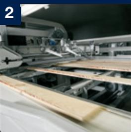
**2** Glue is applied to the edge of the wane timber. Leaving the glue applicator, the lamellas are cross conveyed into a magazine in which they are gathered in a charge.
