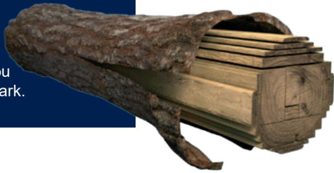
These parts often have wane edges and can be conical and therefore not easily used in conventional production systems.
