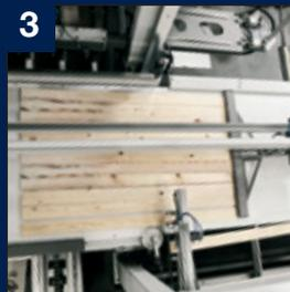
**3** The glued lamellas are fed into the fully automatic press which consists of two parts: a high/radio frequency unit and a hot press unit. The high/radio frequency energy targets the moisture in the glue which quickly heats up and cures from the inside. The hot press unit cures the surface of the board, and the process results in a full-through cured board in the shortest cycle time.
