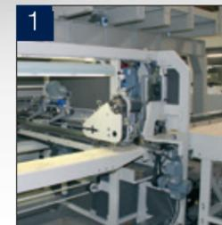
The lamellas pass through the glue applicator one by one. The glue is applied either on top of the lamella by means of a glue nozzle or on the side of the lamella by means of a glue roller, depending on the chosen solution – which again depends on the lamella dimension and your needs.
