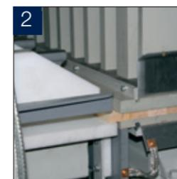
Leaving the glue applicator, the lamellas are cross conveyed into a magazine in which they are gathered in a charge. When the magazine is full, the lamellas are led to a feeding table in front of the press.
